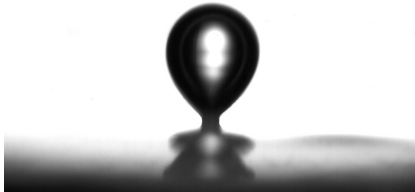
Figure 5.4: Bubble at detachment
