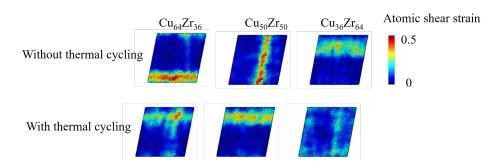
Figure 5.19: Map of the atomic shear strain in the three compositions previously submitted or not to thermal cycling, at 20 % shear strain.
