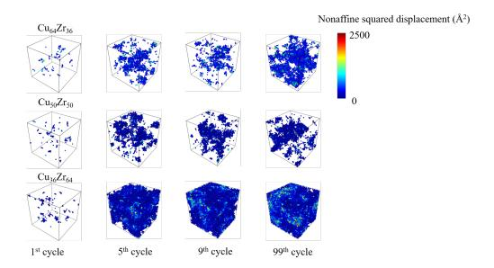
Figure 5.16: Map of the distribution of the non-affine square displacement  $(D_{min}^2 > 100 \text{Å}^2)$  at the 1st, 5th, 9th and 99th cycle, which the previous cycle is the reference for the three studied compositions.
