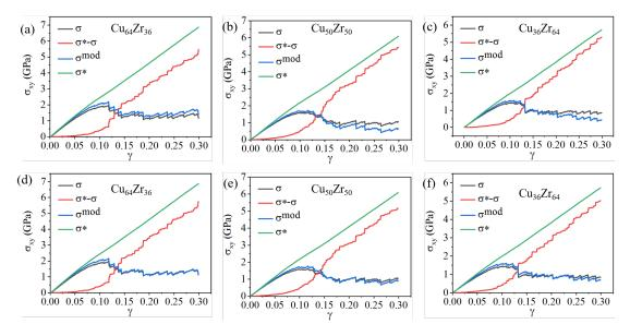
Figure 4.16: The fitting stress-strain curves of three compositions after quenched with quenching rate  $10^{11}$  K/s before correction ((a), (b) and (c)) and after correction ((d), (e) and (f)).
