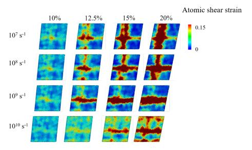
Figure 3.25: Distribution of atomic shear strain of  $Cu_{64}Zr_{36}$  MGs with different strain rates, at strain 10 %, 12.5 %, 15 %, and 20 %, at 0.1 K.
