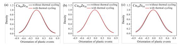
Figure 5.24: Orientation distribution (gaussian fit) of the plastics events occurring over the whole shearing test for each composition before and after thermal cycling.
