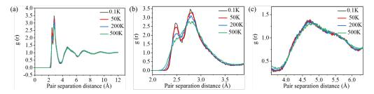
Figure 3.28: The total RDF of  $Cu_{64}Zr_{36}$  MG at different temperatures for quenching rate  $10^{11}$  K/s (a), magnified first peak (b) and magnified second peak (c).
