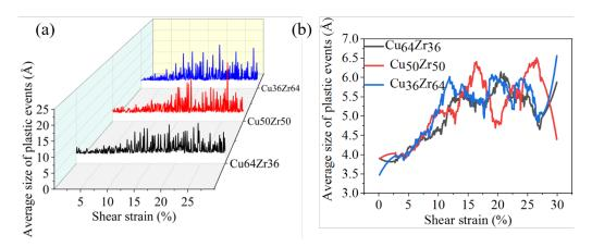
Figure 4.12: Average size of plastic events as a function of the shear strain for the three compositions (a) and the curves after smoothed with SG filter method (b).
