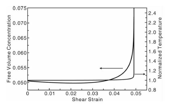
Figure 1.15: Evolution of free volume and temperature during the shear localization process.
