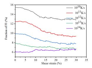
Figure 3.10: Fraction of FI of  $Cu_{64}Zr_{36}$  prepared with different quenching rates as a function of shear strain at 0.1 K.
