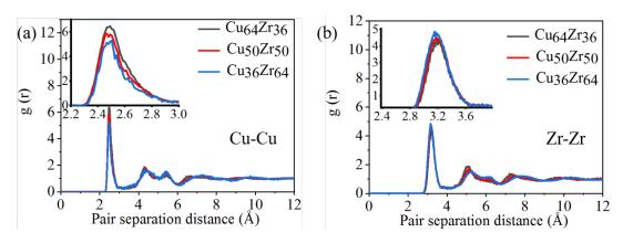
Figure 3.14: Cu-Cu (a) and Zr-Zr (b) partial radial distribution function (PRDF) for three compositions of binary Zr-Cu MGs quenched at 0.1 K at a quenching rate of 10<sup>11</sup> K/s. The insets in the Figures show a magnification of the first peaks.
