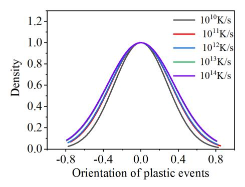
Figure 4.7: Distribution of orientation of all the plastic events occurring during a shear test of  $Cu_{64}Zr_{36}$  MG quenched at different quenching rates.
