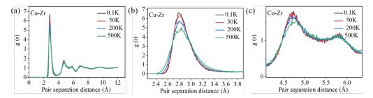
Figure 3.30: The Cu-Zr PRDF of  $Cu_{64}Zr_{36}$  MG at different temperatures for quenching rate  $10^{11}$  K/s (a), magnified first peak (b) and magnified second peak (c).
