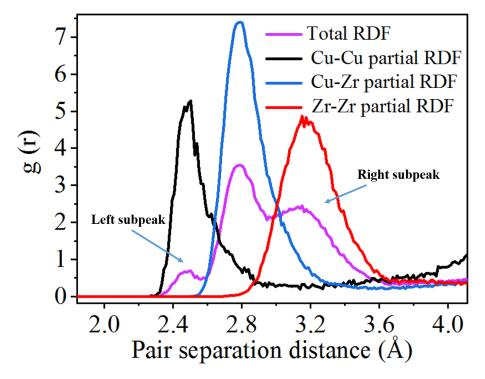
Figure 3.5: The first peak on RDF and partial RDF of  $Cu_{36}Zr_{64}$  MG after quenching with a quenching rate of  $10^{10}$  K/s at 0.1 K.
