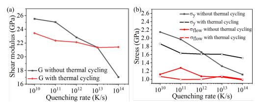
Figure 5.6: Shear modulus (a), yield stress and flow stress (b) of  $Cu_{64}Zr_{36}$  MG quenched at different initial quenching rates with and without thermal cycling.
