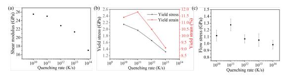
Figure 3.7: Shear modulus (a), yield stress and strain (b), and flow stress (c) for  $Cu_{64}Zr_{36}$  prepared with different quenching rates.
