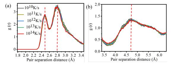
Figure 3.3: The first peak (a) and the second peak (b) on the RDF curves of  $Cu_{64}Zr_{36}$  MG at 0.1 K under different quenching rates.
