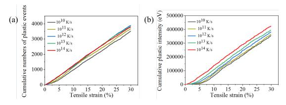
Figure 4.20: Cumulative number (a) and cumulative plastic intensity (b) of plastic events of  $Cu_{64}Zr_{36}$  MG after tensile deformation with different quenching rates.
