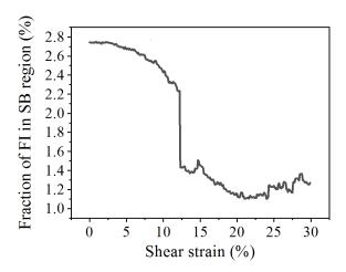
Figure 3.11: Fraction of FI in SB region of  $Cu_{64}Zr_{36}$  prepared with the quenching rate  $10^{10}$  K/s as a function of shear strain.
