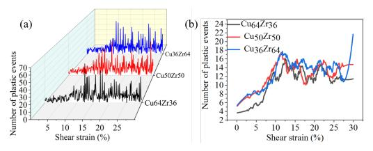
Figure 4.13: *Number of plastic events as a function of the shear strain for the three compositions (original curves (a) and smoothed one with SG filter method (b)).*
