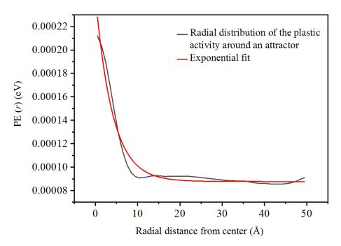
Figure 2.6: Radial distribution of plastic energy PE(r) around the attractor and exponential fit curve [Albaret et al., 2016].
