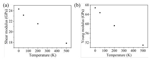
Figure 3.33: Shear modulus (a) and Young's modulus (b) of  $Cu_{64}Zr_{36}$  MG deduced form shear tests and tensile tests at different temperatures and strain rate  $10^8$  s<sup>-1</sup>.
