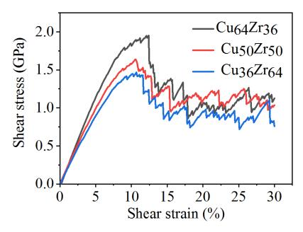
Figure 3.16: Shear stress-strain curves of three compositions quenched at 0.1 K after quasi-static deformation at a quenching rate of  $10^{11}$  K/s.
