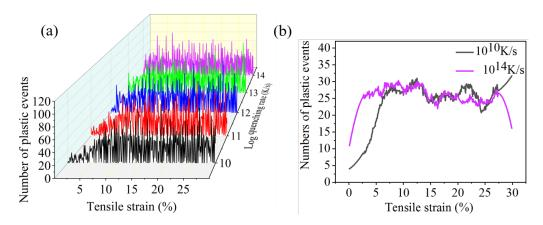
Figure 4.21: Number of plastic events as a function of the tensile strain for  $Cu_{64}Zr_{36}$  MG quenched at different quenching rates (a) and smoothed curve for quenching rate  $10^{10}$  K/s and  $10^{14}$  K/s (b).
