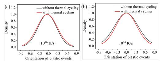
Figure 5.14: Distribution of orientation of plastic events of  $Cu_{64}Zr_{36}$  MG without and with thermal cycling for quenching rate of  $10^{10}$  K/s (a) and a quenching rate of  $10^{14}$  K/s (b).
