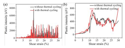
Figure 5.12: Plastic intensity of plastic events of  $Cu_{64}Zr_{36}$  MG (initial quenching rate  $10^{10}$  K/s) without and with thermal cycling (a) and smoothed curves (b).
