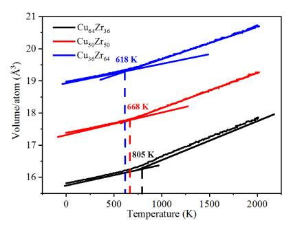
Figure 3.12: Volume as a function of the temperature for the three different compositions quenched with a quenching rate of  $10^{11}$  K/s. Dotted lines are to determine the glass transition temperature.
