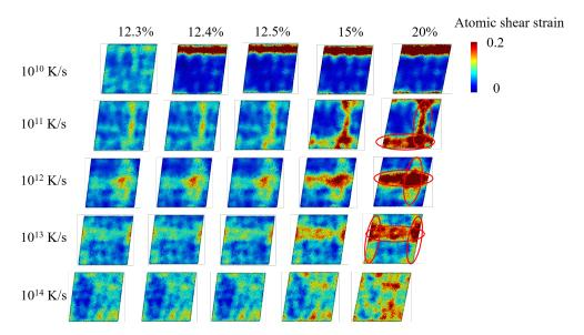
Figure 3.9: The atomic shear strain in  $Cu_{64}Zr_{36}$  MG prepared with different quenching rates at different shear strains, at 0.1 K.
