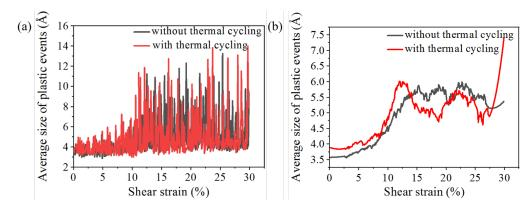
Figure 5.8: Comparison of average size of plastic events of  $Cu_{64}Zr_{36}$  MG (initial quenching rate  $10^{10}$  K/s) without and with thermal cycling (a) and smoothed curves (b).
