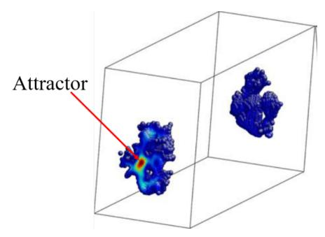
Figure 2.5: Map of plastic energy, PE(r) surrounding a plastic event (the intensity of plastic energy from low to high) corresponding to the color from blue to red [Fusco et al., 2010].
