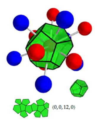
Figure 1.7: <0,0,12,0> icosahedron in  $Cu_{64}Zr_{36}$  metallic glass.
