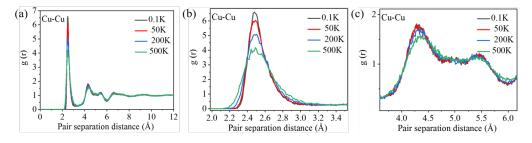
Figure 3.29: The Cu-Cu PRDF of  $Cu_{64}Zr_{36}$  MG at different temperatures for quenching rate  $10^{11}$  K/s (a), magnified first peak (b) and magnified second peak (c).
