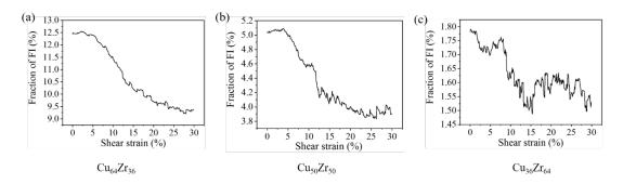
Figure 3.21: Comparison of fraction of FI with shear strain for the three compositions.
