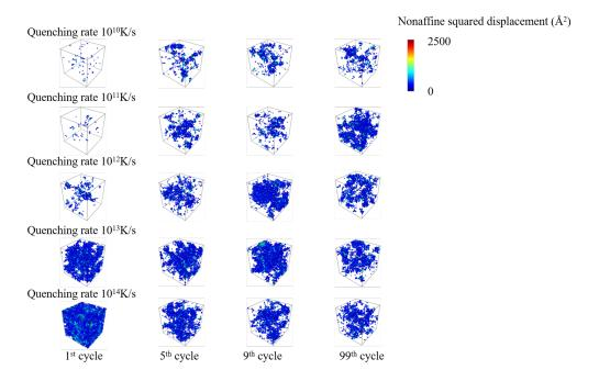
Figure 5.4: Map of the distribution of the non-affine square displacement ( $D_{min}^2 > 100 \text{Å}^2$ ) at the 1st, 5th, 9th and 99th cycle, calculated with the previous cycle as reference, for  $Cu_{64}Zr_{36}$  MGs prepared with different quenching rates.
