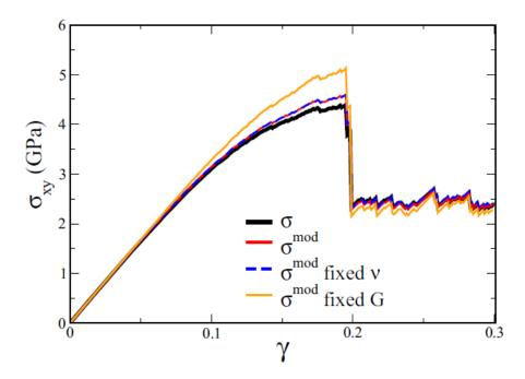
Figure 1.19: Comparison of shear stress-strain curves for amorphous silicon with Stillinger and Weber (SW) potential [Stillinger and Weber, 1985] from MD simulations and with Eshleby's inclusion model. The black curve is the result of the MD simulation. Red, dashed blue and orange curves are obtained with Eshelby's inclusion model [Albaret et al., 2016].
