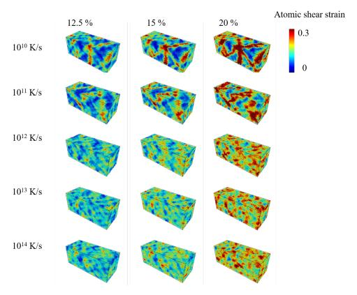
Figure 4.24: Map of the atomic shear strain for tensile strain 12.5 %, 15 % and 20 % for  $Cu_{64}Zr_{36}$  MG quenched at different quenching rates.
