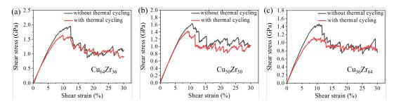
Figure 5.17: *Stress-strain curves in quasi static shear for the three compositions previously submitted or not to the complete thermal cycling.*
