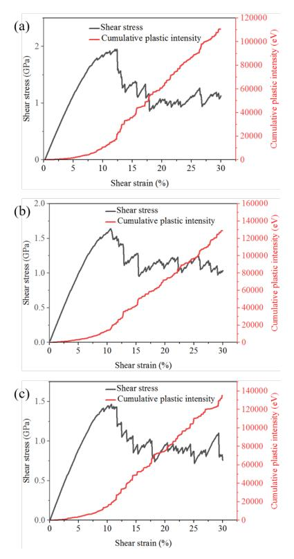
Figure 4.11: Shear stress and cumulative plastic intensity as a function of the shear strain for the three compositions,  $Cu_{64}Zr_{36}$  (a),  $Cu_{50}Zr_{50}$  (b), and  $Cu_{36}Zr_{64}$  (c).
