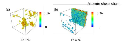
Figure 3.8: Map of atomic shear strain in  $Cu_{64}Zr_{36}$  MG prepared with a quenching rate of  $10^{10}$  K/s, sheared at 12.3 % strain (a) and 12.4 % (b), showing the atoms with shear strain larger than 60 % of the maximum atomic shear strain over the whole sample.
