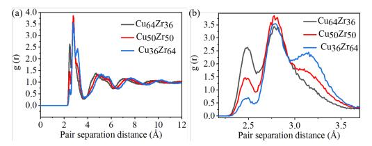
Figure 3.13: The total radial distribution function (RDF) for three compositions of binary Cu-Zr MGs quenched at 0.1 K at a quenching rate of  $10^{11}$  K/s (a) and the magnification of the first peak (b).
