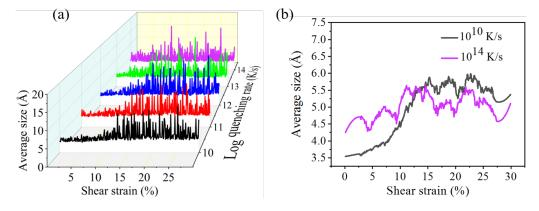
Figure 4.6: Comparison of the average size of plastic events with strain for different quenching rates (a) and comparison between quenching rates  $10^{10}$  K/s and  $10^{14}$  K/s after smoothing with SG filter method (b).
