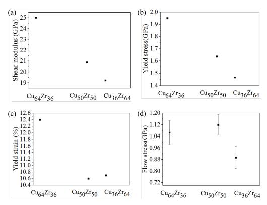
Figure 3.17: Shear modulus (a), yield stress (b), yield strain (c) and flow stress (d) of three compositions quenched at 0.1 K at a quenching rate of  $10^{11}$  K/s.
