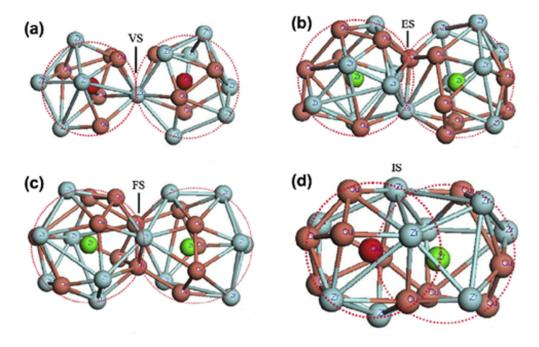
Figure 1.9: SRO clusters connected by (a) VS, (b) ES, (c) FS, and (d) IS in the  $Cu_{50}Zr_{50}$  metallic glass (Zr and Cu atoms are represented with blue and brown balls, respectively, and centered Zr and Cu atoms are represented using green and red balls, respectively) [Li et al., 2014].
