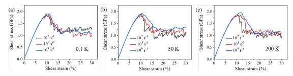
Figure 3.26: Comparison of stress-strain curves of  $Cu_{64}Zr_{36}$  MGs sheared with different strain rates, at three different temperatures: (a) 0.1 K, (b) 50 K, (c) 200 K.
