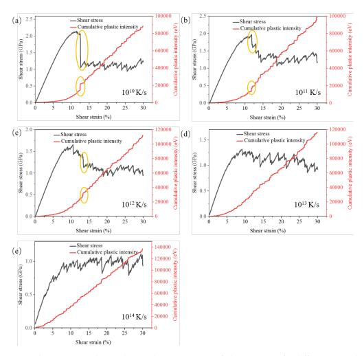
Figure 4.3: *Shear stress and cumulative plastic intensity of plastic events for different quenching rates.*
