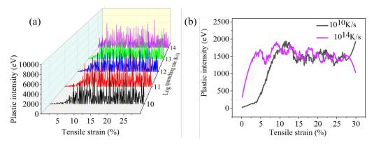
Figure 4.22: Plastic intensity of plastic events as a function of the tensile strain for  $Cu_{64}Zr_{36}$  MG quenched at different quenching rates (a), smoothed curve for quenching rate  $10^{10}$  K/s and  $10^{14}$  K/s (b).
