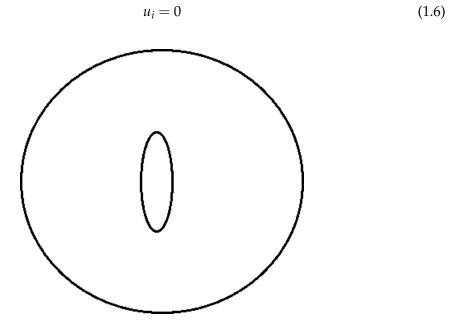
Figure 1.18: Releasing the surface traction of the inclusion.
