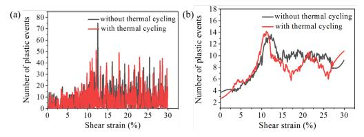
Figure 5.10: Number of plastic events of  $Cu_{64}Zr_{36}$  MG (initial quenching rate  $10^{10}$  K/s) without and with thermal cycling (a) and smoothed curves (b).
