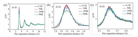
Figure 3.31: The Zr-Zr PRDF of  $Cu_{64}Zr_{36}$  MG at different temperatures for quenching rate  $10^{11}$  K/s (a), magnified first peak (b) and magnified second peak (c).
