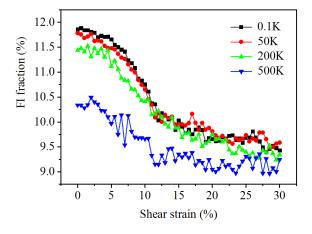
Figure 3.35: Fraction of FI of  $Cu_{64}Zr_{36}$  MG quenched at different temperatures and sheared at the same temperature with a  $10^8$  s<sup>-1</sup> shear strain rate.
