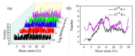
Figure 4.4: Numbers of plastic events as a function of the shear strain, for  $Cu_{64}Zr_{36}$  MG, for different quenching rates (a) and comparison between quenching rates  $10^{10}$  K/s and  $10^{14}$  K/s after smoothing with SG filter method (b).
