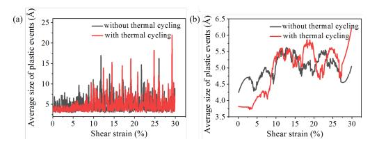
Figure 5.9: Comparison of average size of plastic events of  $Cu_{64}Zr_{36}$  MG (initial quenching rate  $10^{14}$  K/s) without and with thermal cycling (a) and smoothed curves (b).
