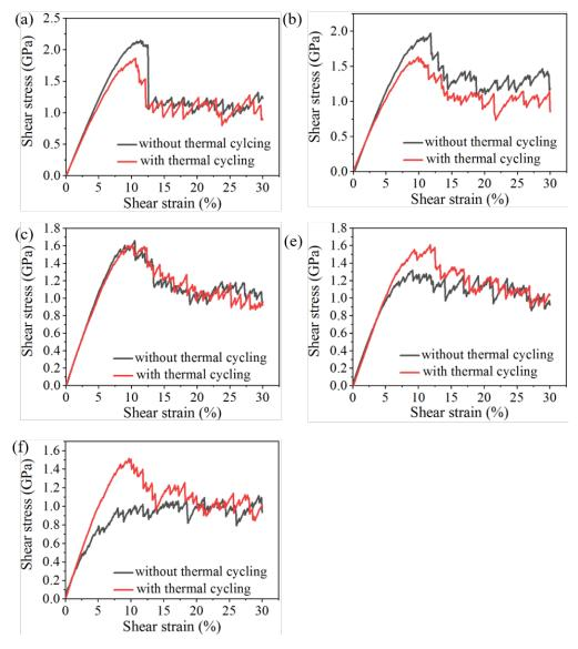
Figure 5.5: Stress-strain curves of  $Cu_{64}Zr_{36}$  MG quenched at different quenching rates ( $10^{10}$  K/s (a),  $10^{11}$  K/s (b),  $10^{12}$  K/s (c),  $10^{13}$  K/s (d) and  $10^{14}$  K/s (e), respectively) and submitted or not to 100 thermal cycles.
