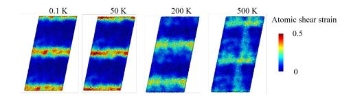
Figure 3.34: Distribution of atomic shear strain at 20 % strain at different temperatures and strain rate  $10^8 \ s^{-1}$  (scale doubled in the y-direction to better visualize).
