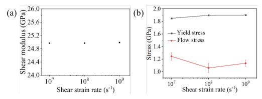
Figure 3.24: Shear modulus (a) and yield and flow stress (b) as a function of the different strain rates for  $Cu_{64}Zr_{36}$  MG quenched at 0.1 K, at a quenching rate of  $10^{11}$  K/s.
