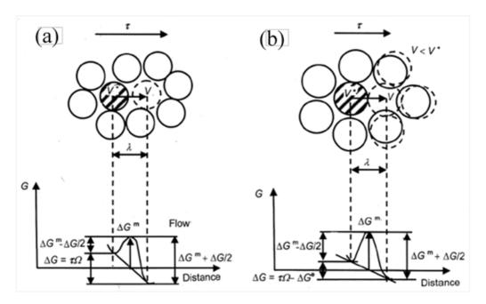
Figure 1.10: Free volume model in the flow of metallic glass [Spaepen, 1977]. (a) Single atomic transition (b) Free volume generation
