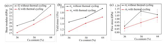
Figure 5.18: Shear modulus G (a), yield stress  $\sigma_y$  (b) and flow stress  $\sigma_f$  (c) deduced from Figure 5.17.
