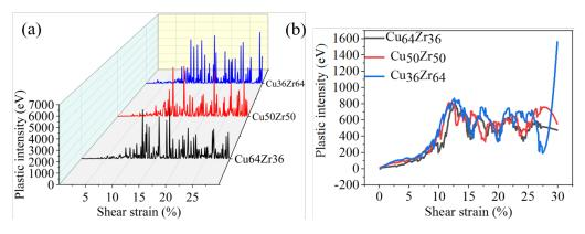
Figure 4.14: Plastic intensity of the plastic events with a function of the shear strain for the three compositions (original curves (a) and smoothed one with SG filter method (b)).
