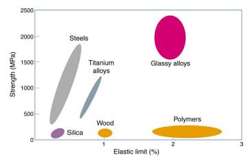
Figure 1.3: Ashby plot of the strength vs. the elastic limit of different classes of materials: amorphous metallic alloys combine the higher strength of crystalline metal alloys with the elasticity of polymers [Telford, 2004].
