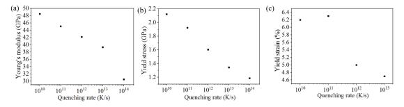
Figure 4.19: Young's modulus (a), yield stress (b) and yield strain (c) of  $Cu_{64}Zr_{36}$  MG for different quenching rates deduced from the tensile stress-strain curve.
