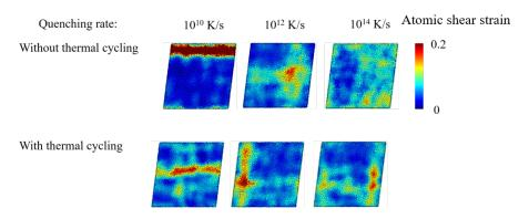
Figure 5.7: Comparison of atomic shear strain of  $Cu_{64}Zr_{36}$  MG quenched at different initial quenching rates with and without thermal cycling, at strain 12.7 %.
