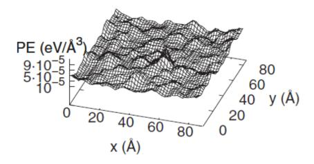
Figure 2.4: 2D projection of density of PE of amorphous silicon over the basins on xy plane at shear strain 1.6 % (40 Å<z<50 Å) [Fusco et al., 2010].
