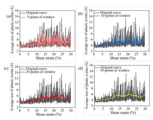
Figure A.2: Different points window of SG filter method when smoothing the curve of average size of plastic events with shear strain of  $Cu_{64}Zr_{36}$  MG with a quenching rate of  $10^{11}$  K/s.
