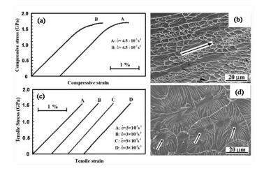
Figure 1.4: Deformation of Zr-based MG in experiment [Zhang et al., 2003]). (a) Compressive strain-stress curve (b) Compression fracture morphology characteristics (c) Tensile strain-stress curve (b) Tensile fracture morphology characteristics
