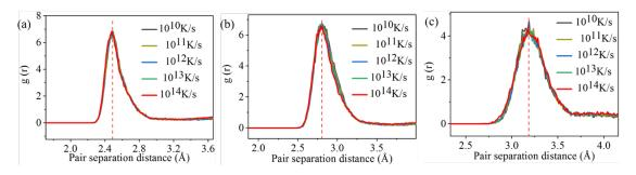
Figure 3.4: The first peaks on Cu-Cu partial RDF curves (a), the first peaks on Cu-Zr partial RDF curves (b), and the first peaks on Zr-Zr partial RDF curves (c) of  $Cu_{64}Zr_{36}$  MG with different quenching rates.
