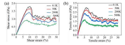
Figure 3.32: Shear stress-strain curves (a) and tensile stress-strain curves (b) of  $Cu_{64}Zr_{36}$  MG at different temperatures and strain rate  $10^8$  s<sup>-1</sup>.
