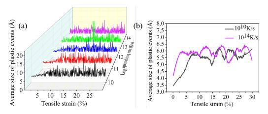
Figure 4.23: Average size of plastic events as a function of the tensile strain for  $Cu_{64}Zr_{36}$  MG quenched at different quenching rates (a) and smoothed curves for  $10^{10}$  K/s and  $10^{14}$  K/s (b).
