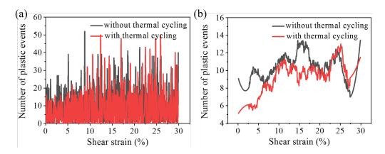
Figure 5.11: Number of plastic events of  $Cu_{64}Zr_{36}$  MG (initial quenching rate  $10^{14}$  K/s) without and with thermal cycling (a) and smoothed curves (b).
