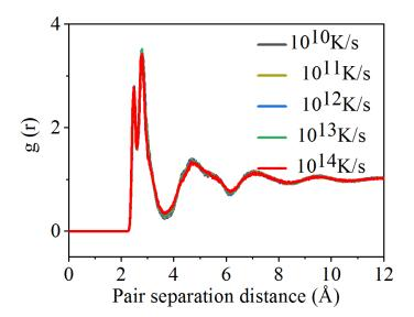
Figure 3.2: Radial distribution function (RDF) of  $Cu_{64}Zr_{36}$  MG at 0.1 K under different quenching rates.
