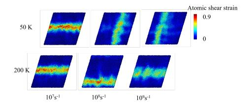
Figure 3.27: Map of atomic shear strain of  $Cu_{64}Zr_{36}$  MG at strain 30 % with strain rate of  $10^7$  s<sup>-1</sup>,  $10^8$  s<sup>-1</sup> and  $10^9$  s<sup>-1</sup> when the temperature is 50 K and 200 K.
