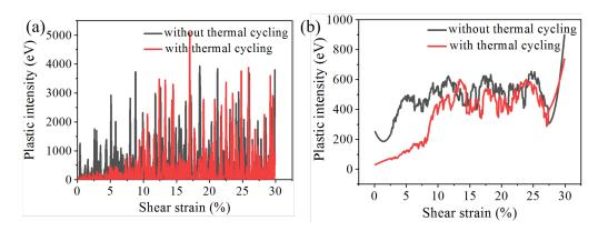
Figure 5.13: Plastic intensity of plastic events of  $Cu_{64}Zr_{36}$  MG (initial quenching rate  $10^{14}$  K/s) without and with thermal cycling (a) and smoothed curves (b).
