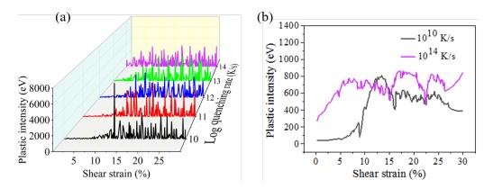
Figure 4.5: Plastic intensity of plastic events for the different quenching rates (a) and comparison between quenching rates  $10^{10}$  K/s and  $10^{14}$  K/s after smoothing with SG filter method (b).
