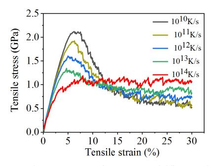
Figure 4.18: Tensile stress-strain curves of  $Cu_{64}Zr_{36}$  MG with different quenching rates.
