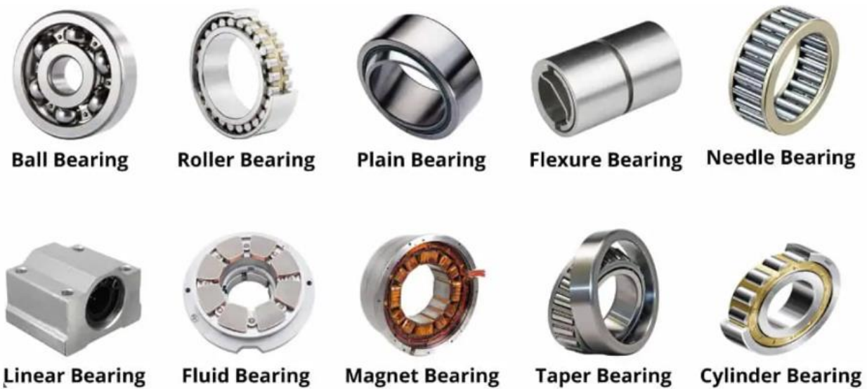
Figure 3.2: Different types de bearings.
