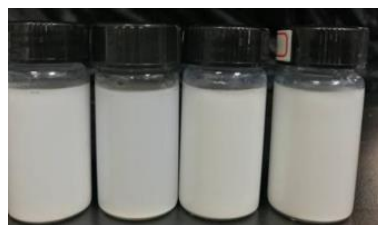
Figure 2.17 : Nano fluid of \text{TiO}_2 in different concentrations [44].
