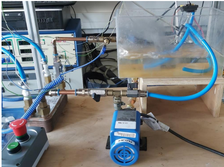
Figure 3.21: Thermo-hydraulic test setup.
