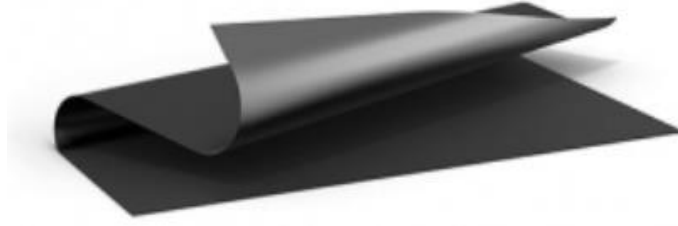
Figure 2.5: Pyrolytic graphite sheet (PGS) [22].
