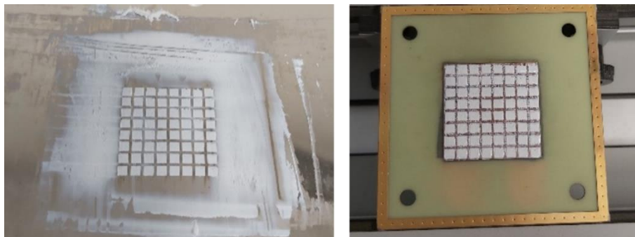
Figure 3.19: Application of the thermal paste on the PCB using a stencil.
