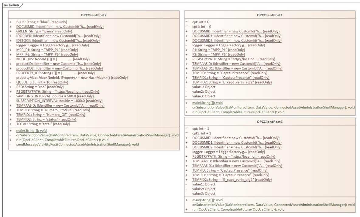
Figure 4.38: Model of OPC clients for stations 1, 6 and 7 of the production line
